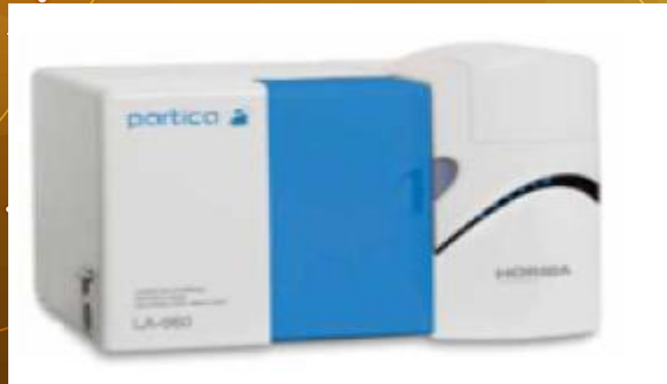
Laser diffraction particle size analysis, Horiba LA-960A
