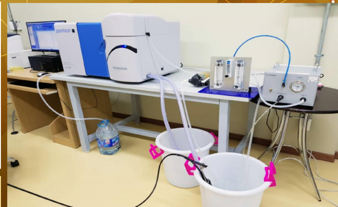
Laser diffraction particle size analysis, Horiba LA-960A
