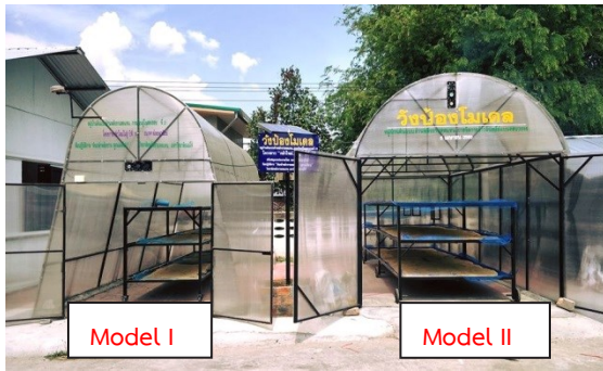
Figure 3 Model I: drying paddy rice in the community by using greenhouse solar dryer with gasified system and Model II: drying paddy rice in the community by using greenhouse solar dryer with direct combustion system
